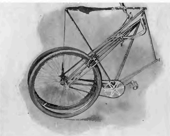
FOLDING TYPE OF CYCLE. Dursley-Pedersen Cycle Co., Ltd., Dursley.
